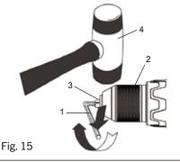
**NOTE:** Turn the screw COUNTER-CLOCKWISE to tighten it. This screw has a left-handed thread.
