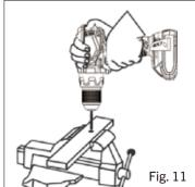
MARNING: Be prepared for binding and bit breakthrough. When these situations occur, the drill bit has a tendency to grab the workpiece. This action will kick the drill opposite to the direction of the drill bit rotation and could cause loss of control when breaking through material as you complete drilling the hole. If you are not prepared, this loss of control can result in serious injury.
