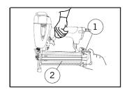
Insert a strip of nails (1) into the magazine. After ensuring that the points of the nails are facing down, close the magazine.
