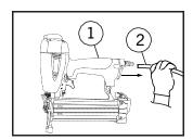
2. Hold the Brad Nailer firmly with one hand, and use the other hand to press the latch (1) on the magazine (2) and slide it back.
